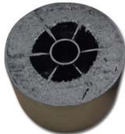
Sectioned Rotor with Contaminant
